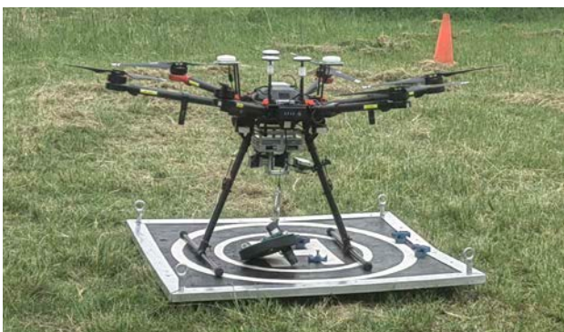
The new technology includes a drone that is fitted with a winch and jig system to house chemical bacterial probes to test for certain quality-related parameters.
