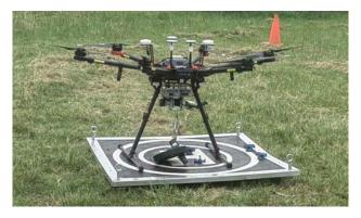
The new technology includes a drone that is fitted with a winch and jig system to house chemical bacterial probes to test for certain qualityrelated parameters.
