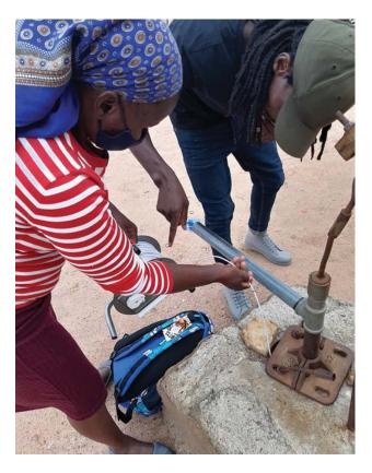
Citizen scientists using a dip meter to measure water levels of boreholes in Limpopo's Hout catchment area.
