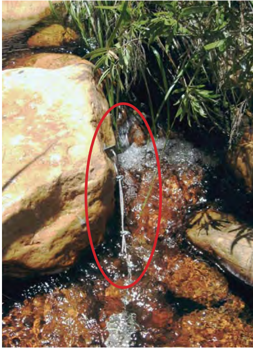
The wire hanging down in the middle of the picture (circled in red) carries a series of tiny thermal probes used to capture a record of water temperature.
