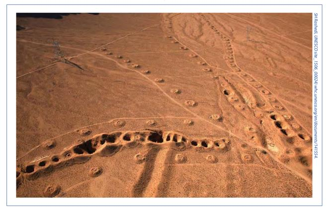
A series of qanats in Iran. The holes surrounded by mounds are vertical chimneys leading to underground water sources. The image shows evidence of at least four separate underground 'rivers'.
