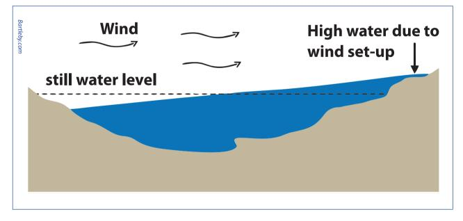
A seiche is essentially a wind-generated internal wave that causes the water surface to slope.
