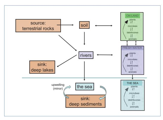
A much simplified phosphorus cycle. See text and box on phosphorus (Chapter 7) for details.
