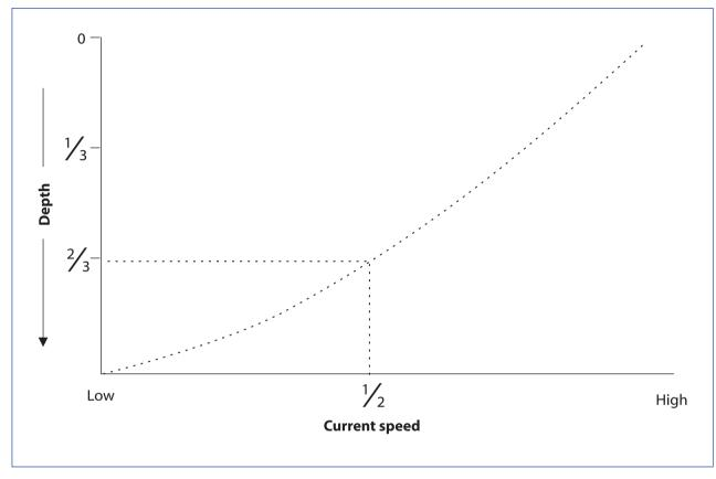
Relationship between current velocity and depth, average velocity occurring at two-thirds of the distance from the surface.
