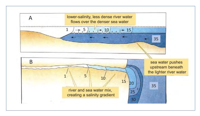
Diagram showing the 'salt wedge' in an estuary caused by less dense river water flowing over denser sea water. A) vertical profile and B) view from above. Numerals refer to salinity values.
