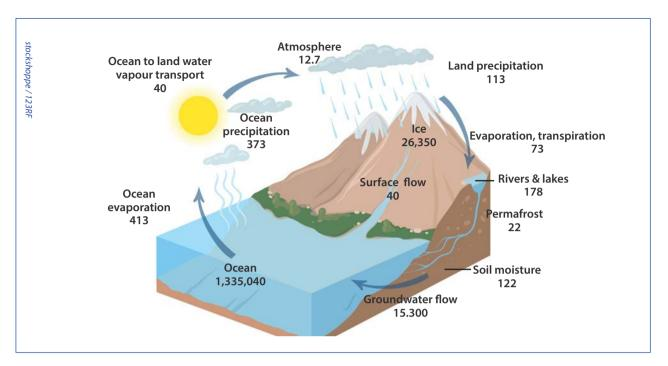
The hydrological cycle: storage of water in thousands of km<sup>3</sup> and fluxes (exchanges) in thousands of km<sup>3</sup> per year.
