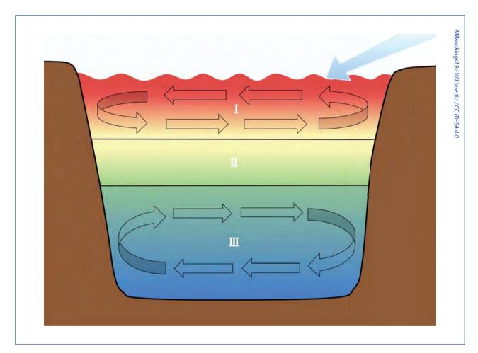
Lake stratification: the warmer epilimnion (red) becomes separated from the cool hypolimnion (blue) by the metalimnion, which is charaterised by a steep temperature gradient known as the thermocline.
