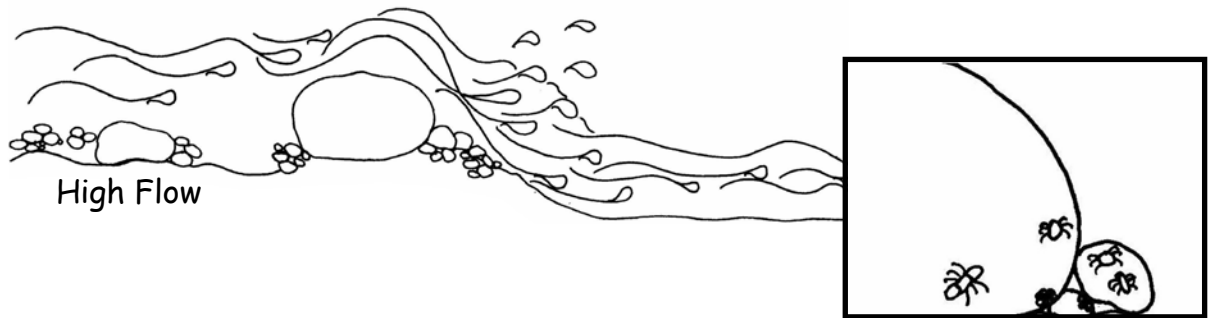
Diagram 12a: How hydraulic biotopes form depends on the shape of sediment materials, and on the flow regime of the river channel. When flow rates (velocity and depth) change, so does habitat.
