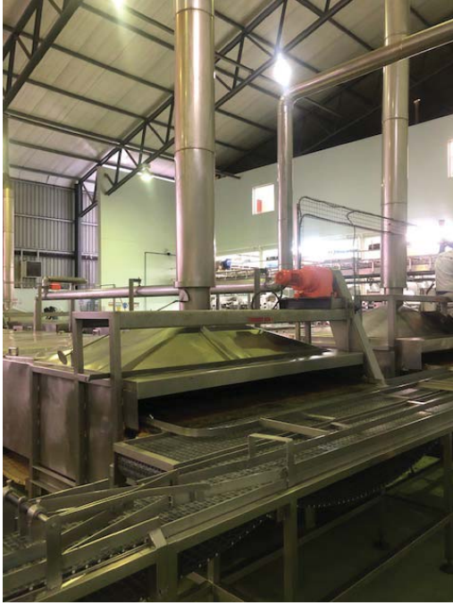
Figure 10-5: Photo Image of a Pre-Cooker at Afro Fishing
