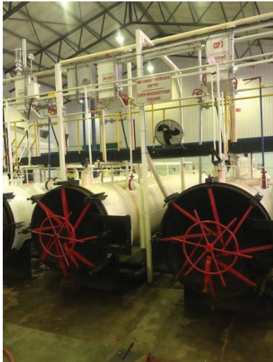
Figure 10-8: Photo Image of Fish Cookers at Afro Fishing
