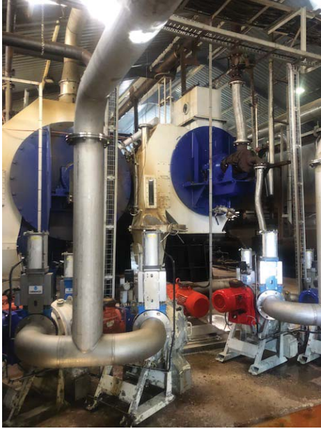
Figure 10-12: Photo Image of Fish Meal Cooker at Lucky Star, St Helena Bay
