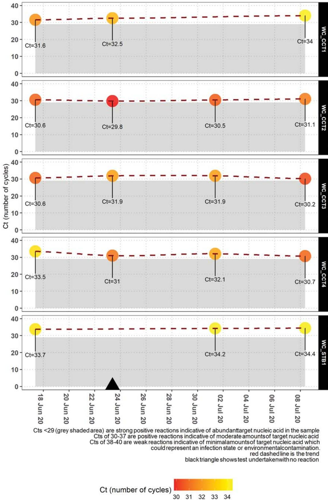
Figure 3-21: Trends in Ct values, by minimum Ct value per site for wastewater treatment works. A black triangle is indicative of a negative result (Ct > 40)
