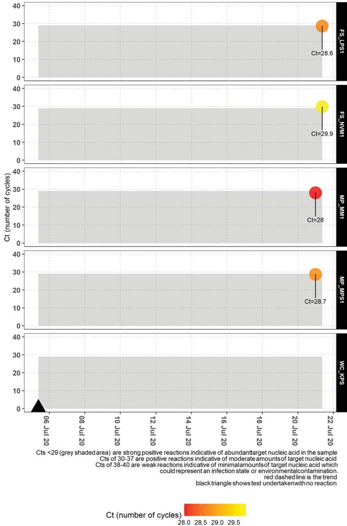
Figure 3-23: Trends in Ct values, by minimum Ct value per site for the power station and mine sites A black triangle is indicative of a negative result (Ct > 40)
