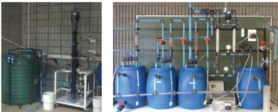
**Figure 5.4:** Pilot plant configuration – Anaerobic Expanded Granular Sludge Bed (EGSB) pre-treatment with downstream MLE AS external MBR
