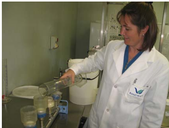
Figure 4.6: Vacuum manifold fitted with 47 mm membrane filter holders.
