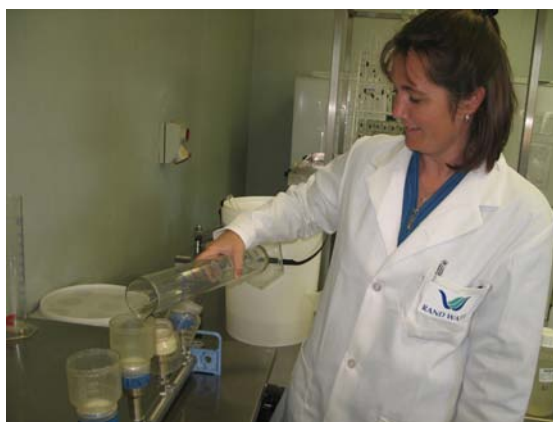
Figure 5.19: Vacuum manifold fitted with 47 mm membrane filter holders.
