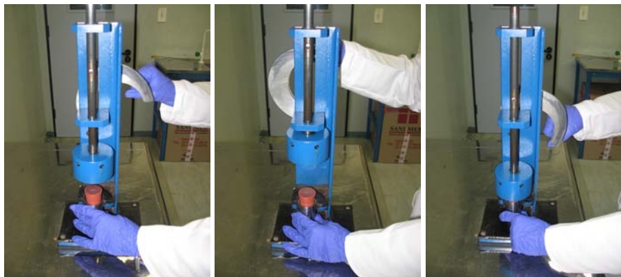
Figure 4.4: Deflation instrument (mechanical hammer), used to disrupt the gas vacuoles of the cyanobacteria, in order for buoyant cells to settle to the bottom of the counting chamber.
