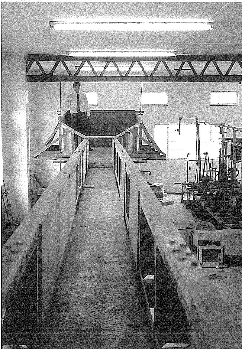
Flume constructed for experiments related to research on sediment-induced density currents (University of Pretoria).
