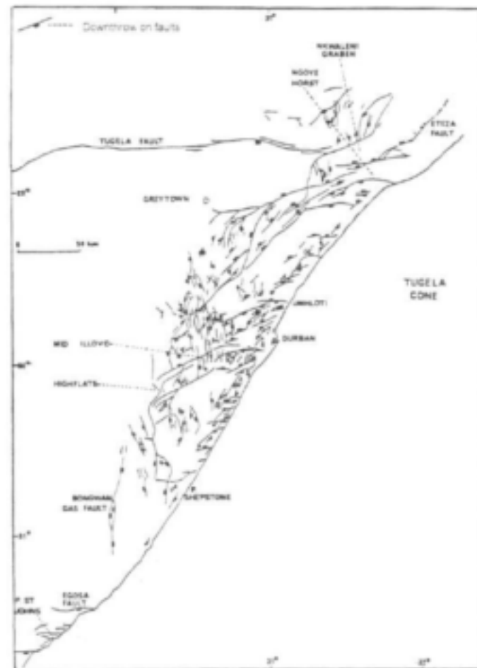
Figure 2-5 Faulting on the coast of KwaZulu-Natal (Martin, 1983).
