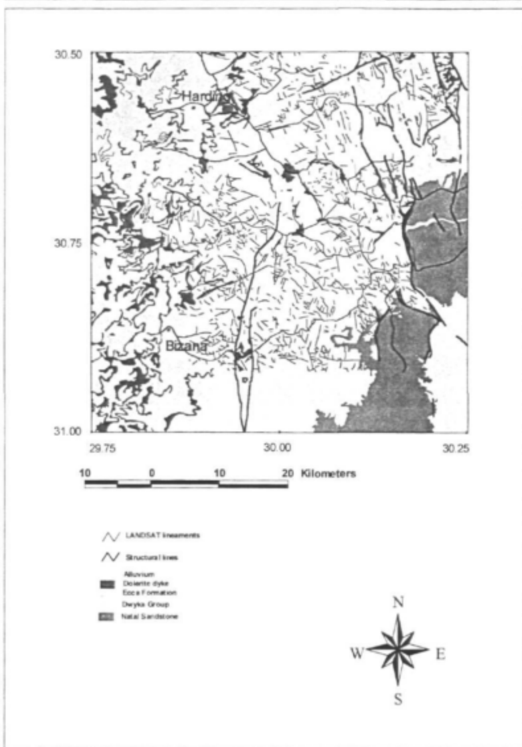
Figure 1-18 Lineament map of the study area on the basis of LANDSAT data
