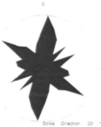
Figure 1-25 Orientation of all joints and faults within the tillite
