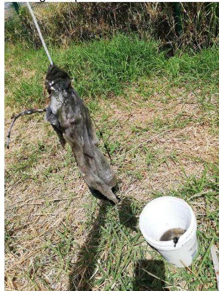
Passive sampler from Black River after 24h deployment
