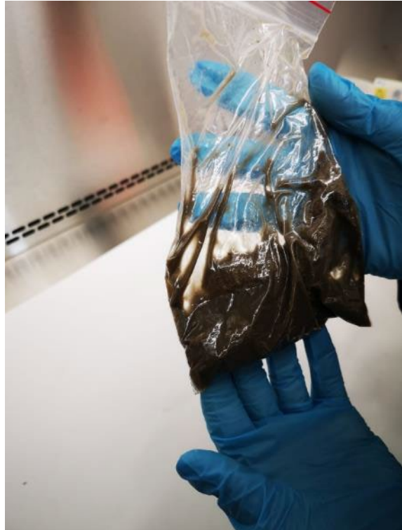
After 48 hours, sample swab is significantly fouled
