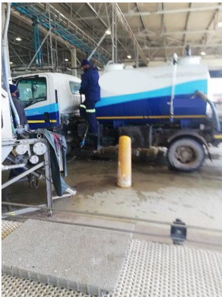
Tanker trucks collecting waste from septic tanks and chemical toilets discharging to the wastewater treatment works
