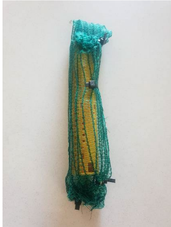
Torpedo filled with gauze and wrapped in shade cloth ready for deployment.
