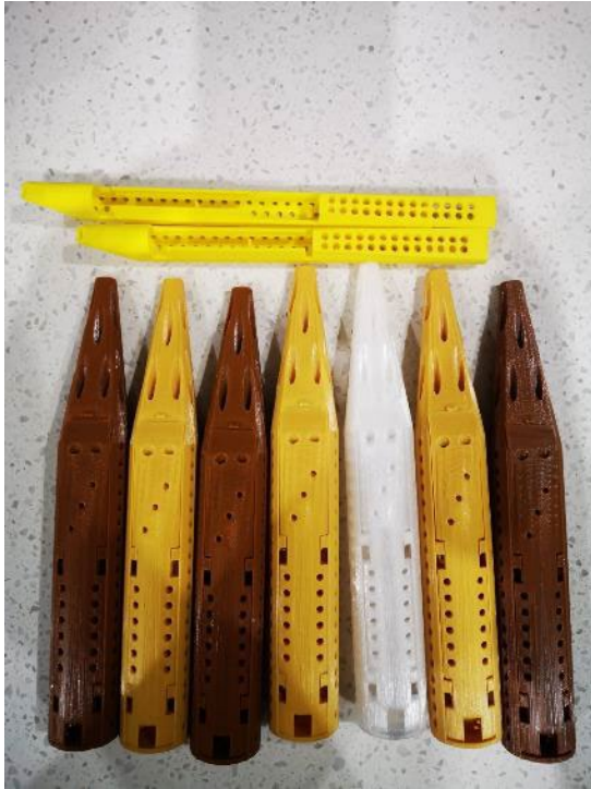
Torpedo style passive sampling devices and two pipe sampling devices (above)
