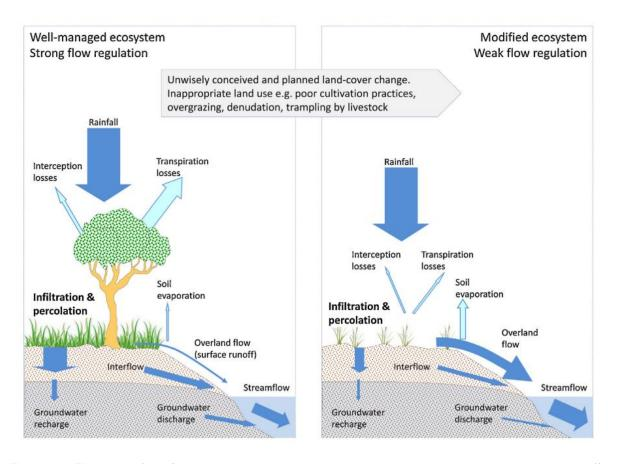
Figure 4-1 Elements of the flow regulation service, the processes that link them and how they are affected by land cover change and inappropriate land use (sourced from Le Maitre, Kotzee and O'Farrell, 2014: p. 173)
