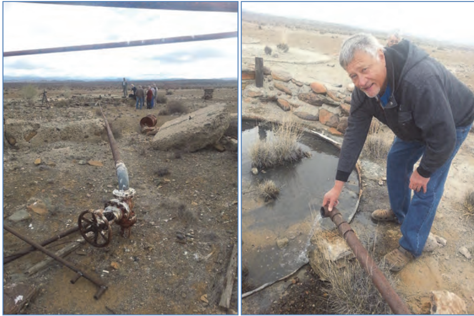
Photos 17 & 18. Borehole SA1/66 and Prof. Van Tonder at the discharge point after opening the flow valve in 2012
