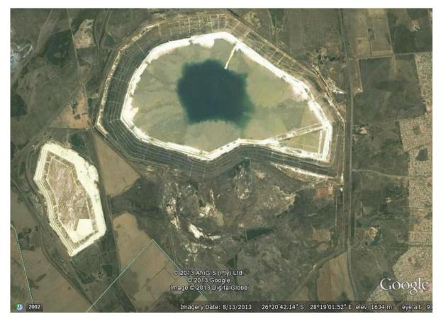
Figure 2 Ergo's Brakpan Dam tailings storage facility south of Brakpan adjoining the Blesbokspruit and the Heidelberg Road. The top of the dam is 3.5 km wide and has an area of about 600 ha. Slurry is still pumped into the facility from a site adjacent to where underground water will be pumped at Grootvlei near Springs.
