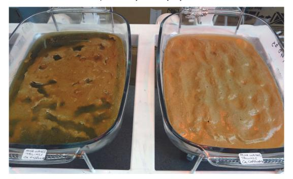
Initial result of mine water addition to tailings limed with Ca(OH)<sub>2</sub> (left) and CaCO<sub>3</sub> (right).
