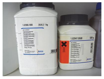
Liming materials used for neutralisation (Ca carbonate and hydroxide)
