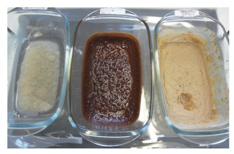
Small basins for mine water neutralisation and evaporation without soil
