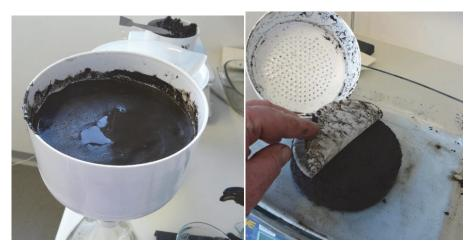
Vacuum extraction of black clay: caking facilitated return to the evaporating basin
