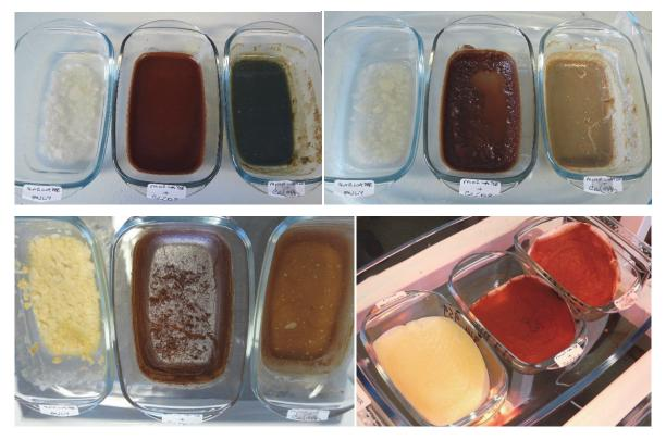
Sequence of residue development during the neutralisation and evaporative concentration of mine water. In each of the four pictures, the basin on the left is untreated mine water, in the middle is neutralised with  $CaCO_3$  and on the right with  $Ca(OH)_2$ . These are treatments OMO, OMC and OMH, respectively, as described in Table A1. The full amount of liming material was added to the basins at the start and the mine water was then added and evaporated daily for twenty days.
