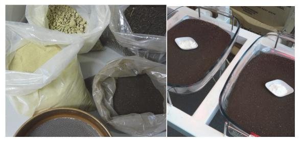
Mine tailings and black clay soil sieved (left) and alkaline treatments applied (right)
