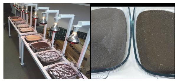
Soil and tailings in evaporation basins with amendments (left) and mixed with lime (right)
