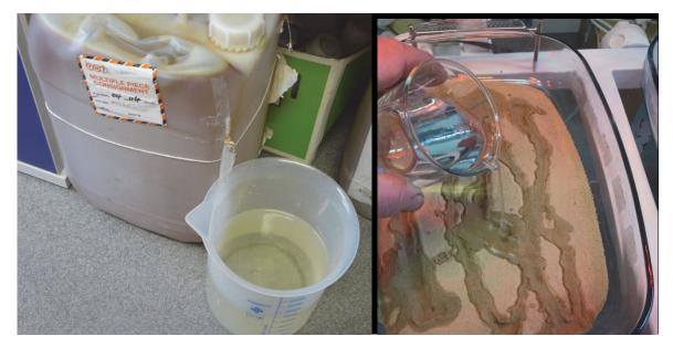
Mine water dispensed from storage tub (left) and added to tailings (right)
