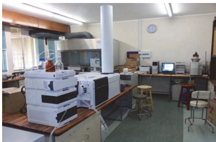
Figure 3.2: The HPLC-QTOF/MS used for the detection of HIV-ARVs in water and fish plasma samples. All calculations were done using MassHunter (Version 5.0) Software (Agilent; Germany).
