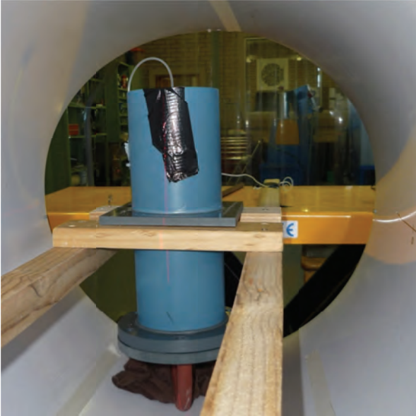
Figure 28. A.) The PET scanner used to follow liquid flow in the PVC column packed with ore shown positioned in the camera. B.) The preliminary result illustrating liquid movement through the ore column. The progression from dark blue (no moisture bearing tracer) to red (high liquid content) demonstrates the non-uniform distribution of the liquid.
