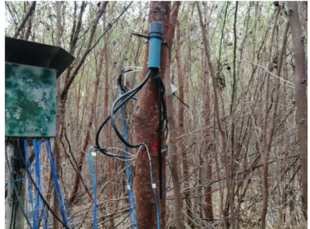
The scientists conducted sap flow measurements to quantify plant water use. They inserted sap flow sensors into the xylem vessels of tree stems. The probes tracked the movement of water through the trees by using heat as a tracer.
