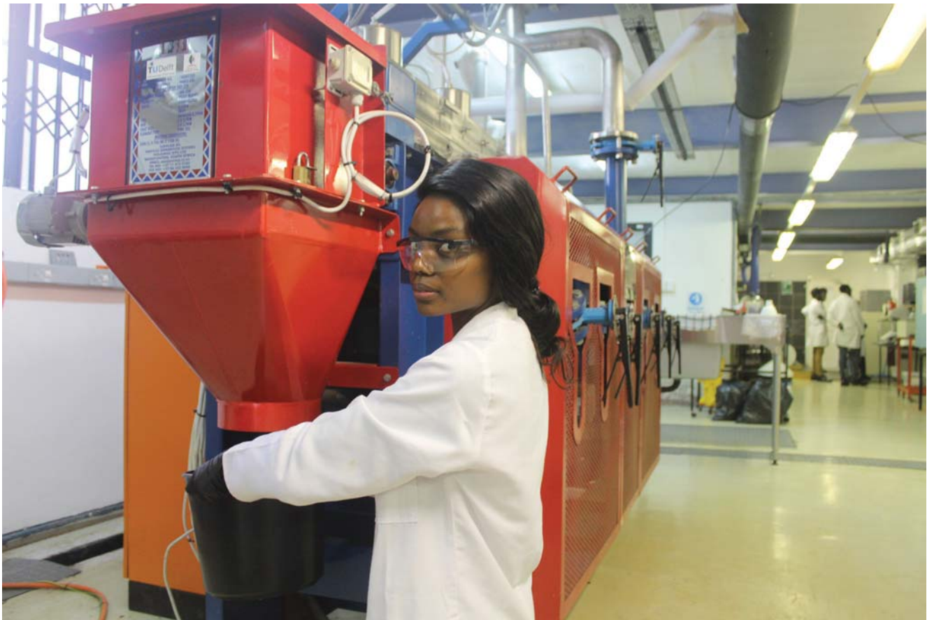
Ncebakazi Ngubane collects dried faecal pellets from a LaDePa machine, a laboratory-scale version of a device which extrudes faecal sludge into pelletised form which is then heated at high temperature to inactivate pathogens.
