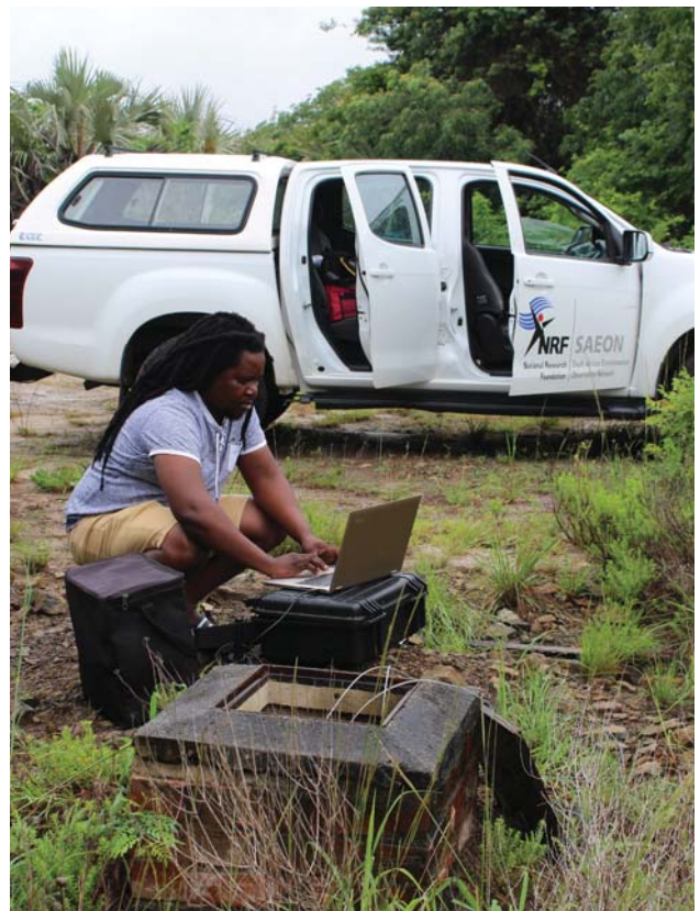
SAEON technician, Sipiwe Mfeka, downloads groundwater data from a monitoring sensor. Working in collaboration with various stakeholders, SAEON has established a network of groundwater monitoring sites which it maintains to determine trends in ground water dynamics and how this links to lake level, climate and different land uses in the region.
