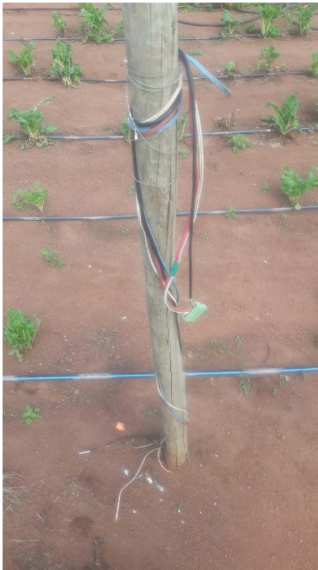
Chameleon sensor at Rooiwal, abandoned and disconnected.
