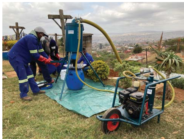
Sani Squad workers use a Pitvaq mobile pit emptying machine to avoid contact with faecal sludge. Groundsheets catch spills, protecting householders and the environment.
