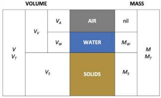
M and V denote mass and volume respectively with the subscripts A. W, S and T referring to air, water, solids and total. Note how gravitational moisture content ratios mass of water to mass of solids, whereas volumetric moisture content relates volume of water to the total or bulk volume.
