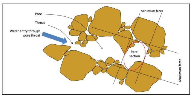
Figure 5-2. Pores, throats and the minimum and maximum Ferret diameters (adapted from Mathews et al. 1997).
