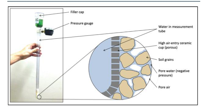
Figure 21-1. Irrometer moisture indicator (left; supplied by CalAfrica) and detail of the ceramic tip of the tensiometer (right; after Lu and Likos 2004).
