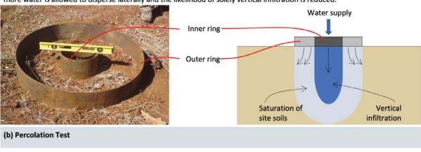
A wide variety of specifications for easy percolation tests from auger holes or shallow excavations are available. Most of these follow interpretation according to Darcy's law and entail the excavation of a test hole with specified dimensions (whether circular to allow excavation by means of hand auger or square to allow excavation by means of shovel). All of these tests are then based on a constant-head or falling-head test in the test hole. The standard set-up is as follows:
