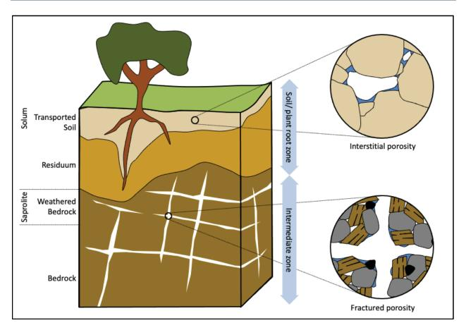
Figure 9-1. Partial saturation of soil and fractured rock.
