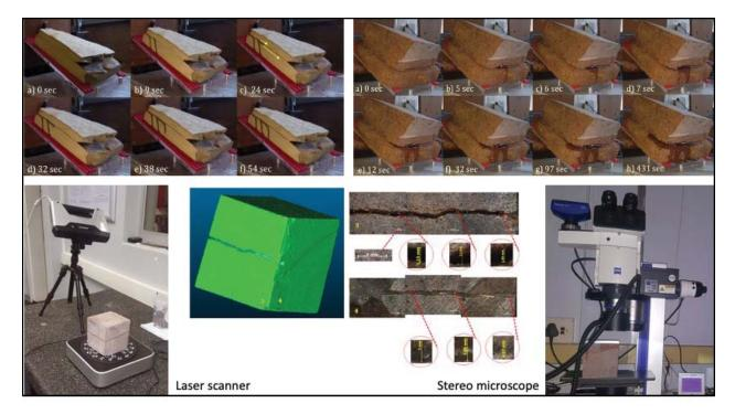
Figure 18-6. VZSA13: Rock specimens inclined at 23°; photography and scanning results to deduce roughness and aperture profiles.
