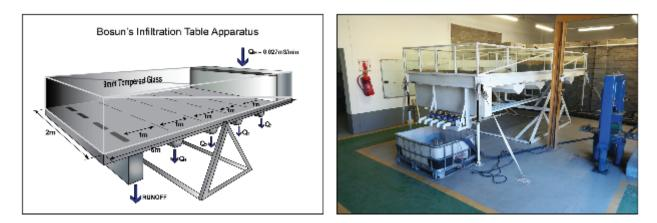
*Figure 20-1. Tilting table schematic construction (left) and final equipment (right); surface area 10 m<sup>2</sup>.*
