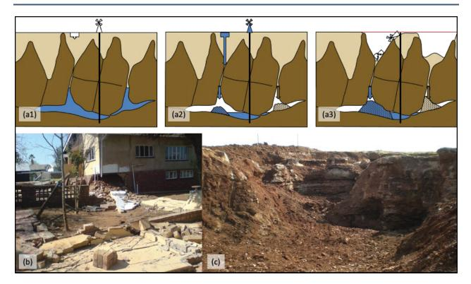
Figure 13-2. (a) Mechanisms of karst-related failure due (Dippenaar et al. 2019a;b); (b) damage to house due to sinkhole (in City of Tshwane in 2012; © MA Dippenaar; (c) sinkhole in Khutsong in shallow dolomite interlayered with chert (3 May 2018; © I Kleinhans).
