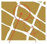
This can also be applied with aerial and linear porosities (as opposed to the volumetric porosity discussed above) with the REV being replaced by the representative elementary area (REA) as the area of investigation is adjusted until porosity stabilizes, or the representative elementary length (REL) as the length of a line through the medium is adjusted until the porosity along the route of the line stabilizes.
