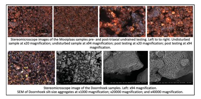
Figure 18-5. VZSA11: Stereomicroscope images of residual dolomite and wad.
