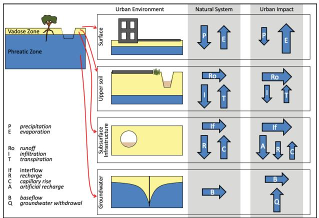
Figure 14-1. Impacts of the urban environment on water balance (arrows indicate modified or newly introduced water flows) (adapted from Schirmer et al. 2013).
