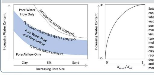
Saturated hydraulic conductivity (i.e. where moisture/ content water = porosity) is the maximum possible value. Different soil types require different moisture contents to enable flow, with clayey soils generally requiring higher degrees of saturation, and sands draining more readily.
