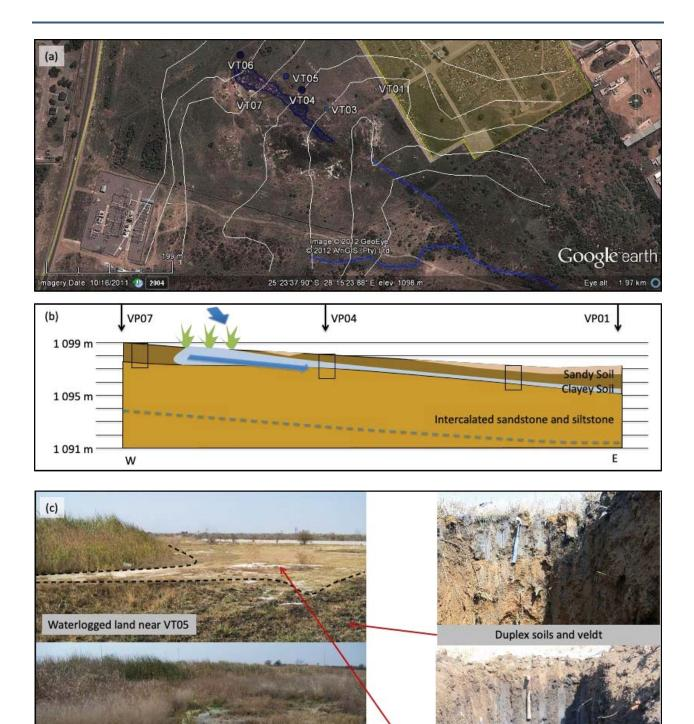
Figure 18-2. VZSA3: (a) Surface elevation, present cemetery (yellow), surface drainage (blue) and sampling positions indicated on Google Earth™ imagery (2013); (b) conceptual model; and (c) view of the site.
