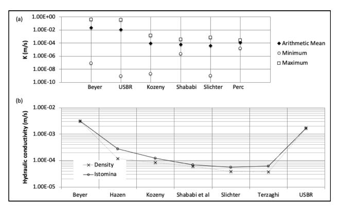
Figure 19-1. Experimental results: empirical grading-based hydraulic conductivities calculated using (a) different approaches and (b) different methods of estimating porosity (Dippenaar et al. 2014; Dippenaar 2014b).
