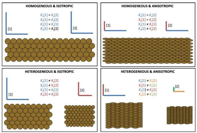
Figure 5-1. Homogeneity and heterogeneity versus isotropy and anisotropy (after Shaw 1994).
