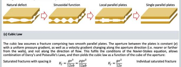
Where  $K_f$  represents the fracture hydraulic conductivity as a function of water's kinematic viscosity (v), dynamic viscosity ( $\mu$ ), density ( $\rho$ ), and gravitational acceleration (g)
