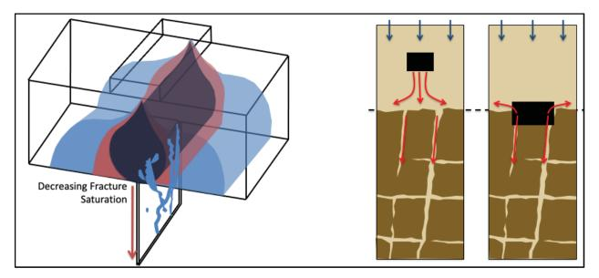
Figure 10-1. Flow along the soil-rock showing the development of a dispersion plume above a fracture (left; Brouwers and Dippenaar 2019), and a scenario where this may occur (right; Dippenaar et al. 2019c).
