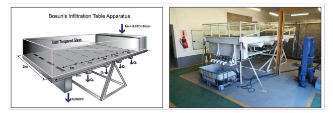
Figure 18-8. VZSA15: Schematic and photograph of the infiltration table apparatus mimicking permeable pavements (Van Vuuren 2020; Van Vuuren et al. 2021).
