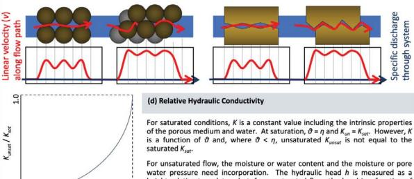
water pressure need incorporation. The hydraulic head h is measured as a height relative to a datum but, for unsaturated flow, the head is a function of the soil suction (or suction head)  $\Psi$  and K is a function of  $\vartheta$ . At a fixed porosity with increasing soil moisture content  $\vartheta$ , the hydraulic conductivity K increases and  $\Psi$  decreases.
