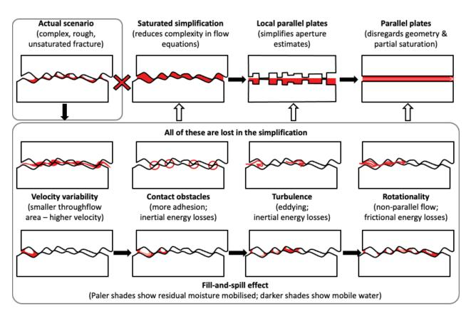
Figure 8-2. Limitations of discreet fracture simplifications (Dippenaar et al. 2020).
