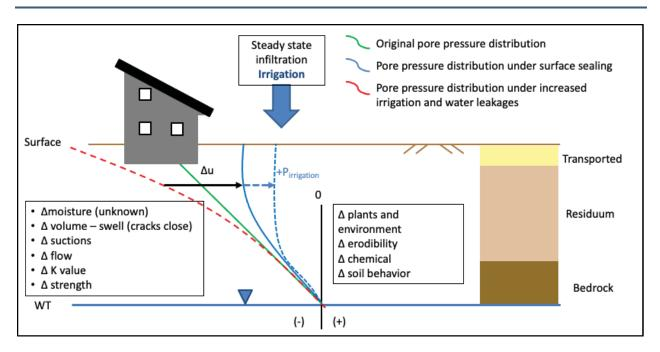
Figure 14-2. Hypothesised influence on subsurface pore water pressure distributions under developments entailing surface sealing and/ or increased water input.
