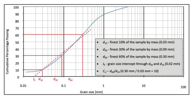
*Figure 3-1.* Determining the d-values from particle size distribution data.
