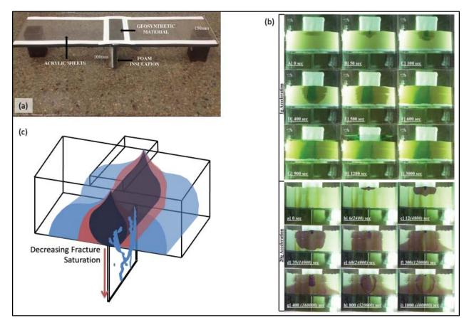
Figure 18-4. VZSA4: (a) Acrylic model of fracture; (b) experimental results showing dispersion in sand overlying single vertical fracture; (c) conceptual model of dispersion and flow mechanisms in fracture.
