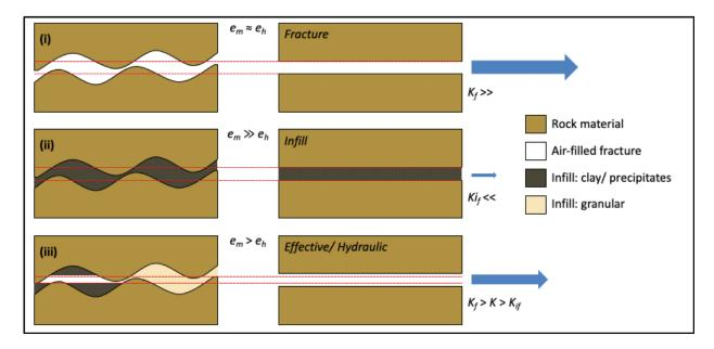
Figure 8-1. Hydraulic ( $e_h$ ) versus mechanical ( $e_m$ ) aperture and resulting fracture ( $K_f$ ), infill ( $K_{if}$ ) and effective overall (K) hydraulic conductivities (Dippenaar and Van Rooy 2016; Jones et al. 2016).
