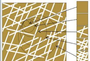
The REV becomes increasingly important when modelling natural systems. As indicated in the instance of a rock mass, different scale of investigation will result in the rock mass being considered as a porous medium; a medium with one discreet or multiple intersecting fractures; a fracture network; and/ or a fracture network behaving again as an equivalent porous continuum.
