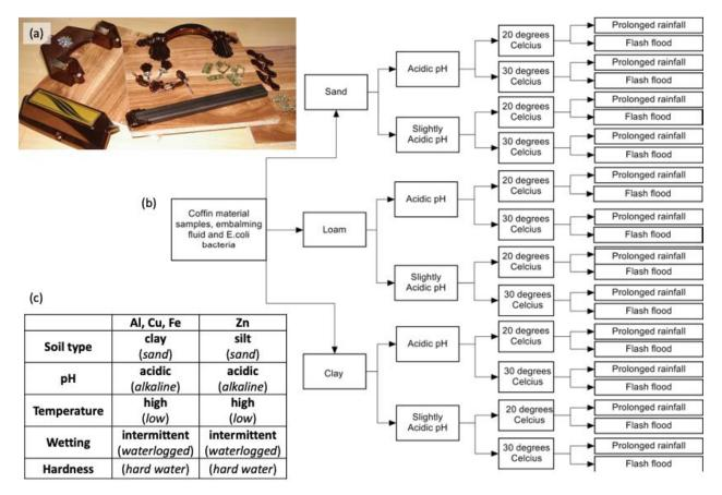
Figure 18-3. VZSA4: (a) Accessory coffin materials tested; (b) experimental planning; (c) key findings (bold - inducing; italics - retarding).
