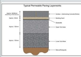
As any road pavement, PICP also has road layers to aid in distribution of the load while, in this instance, allowing drainage of infiltrated water. The natural subgrade (in situ mate will, however, dictate whether deeper percolation can occur at expense of induced lateral interflow.
