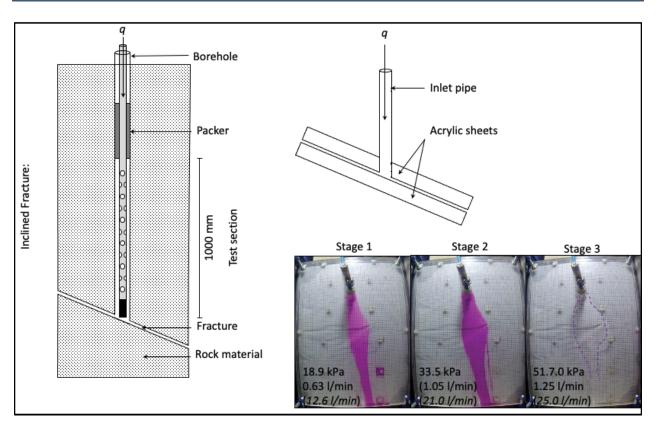
Figure 18-7. VZSA14: Acrylic model as constructed; flow over time at different pressures and fluxes (potassium permanganate used to make flow visible).
