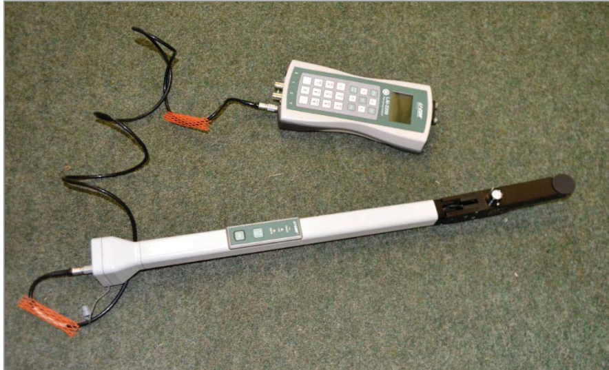
Figure 5.15 LAI-2200 Plant Canopy Analyzer used to measure the average Leaf Area Index (LAI) for the riparian vegetation
