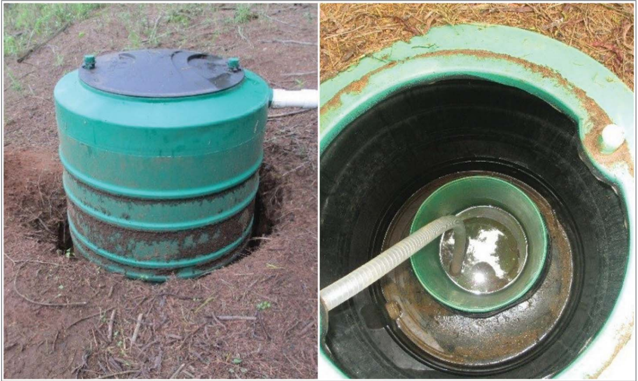
Figure 5.4 JOJO tank gathers the sample (left) and fills the bucket below the runoff plot (right)
