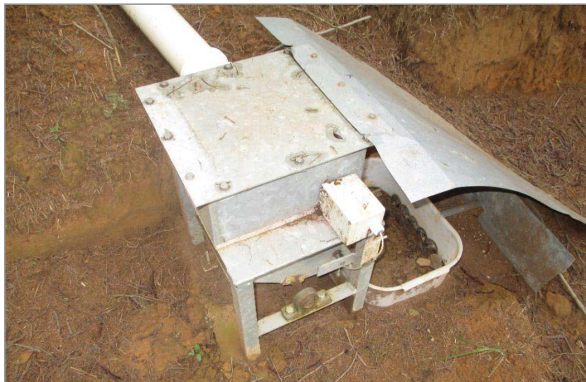
Figure 5.5 Tipping bucket connected to a hobo logger to measure amount of runoff
