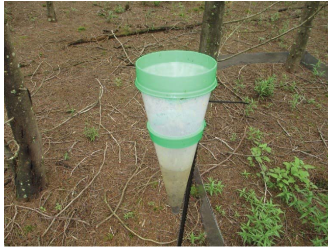
Figure 5.1 Manual rain gauge to measure the amount of rainfall hitting the ground
