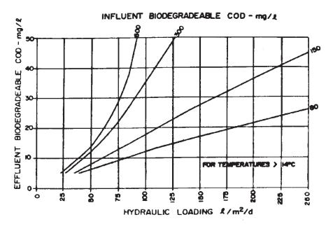
The wetted area is shown as a function of influent and effluent COD in Figure C-1.
