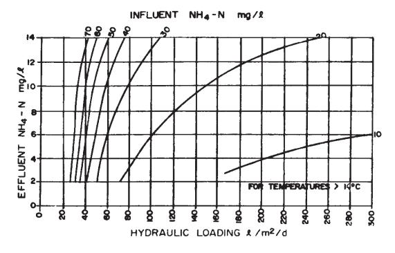
Figure C-2 can be used for design to remove ammonia.
