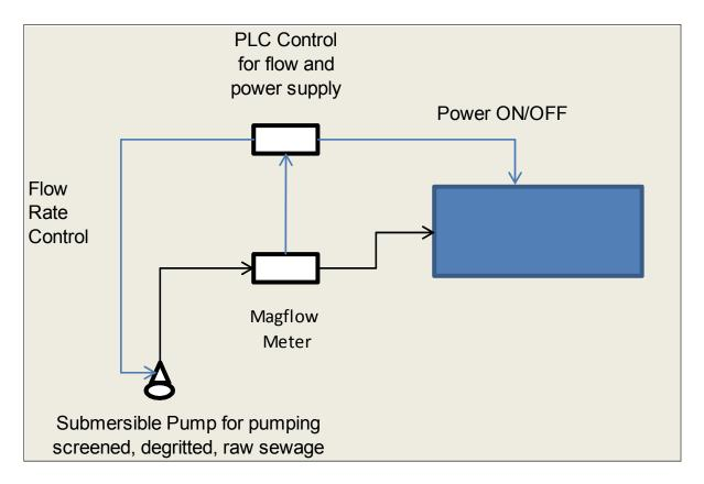
Figure 2-2: Control circuitry for SWWTW Evaluation Facility
