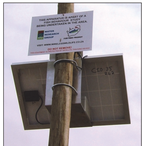
Figure 4: Photograph of a notice board used to deter theft/vandalism of remote stations.
