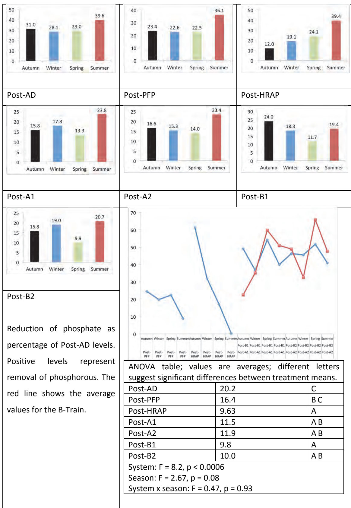
Figure 1.5 Change of phosphate concentration (mg/L) in the effluent as percentage of Post-AD levels. Positive levels represent removal of phosphorous.
