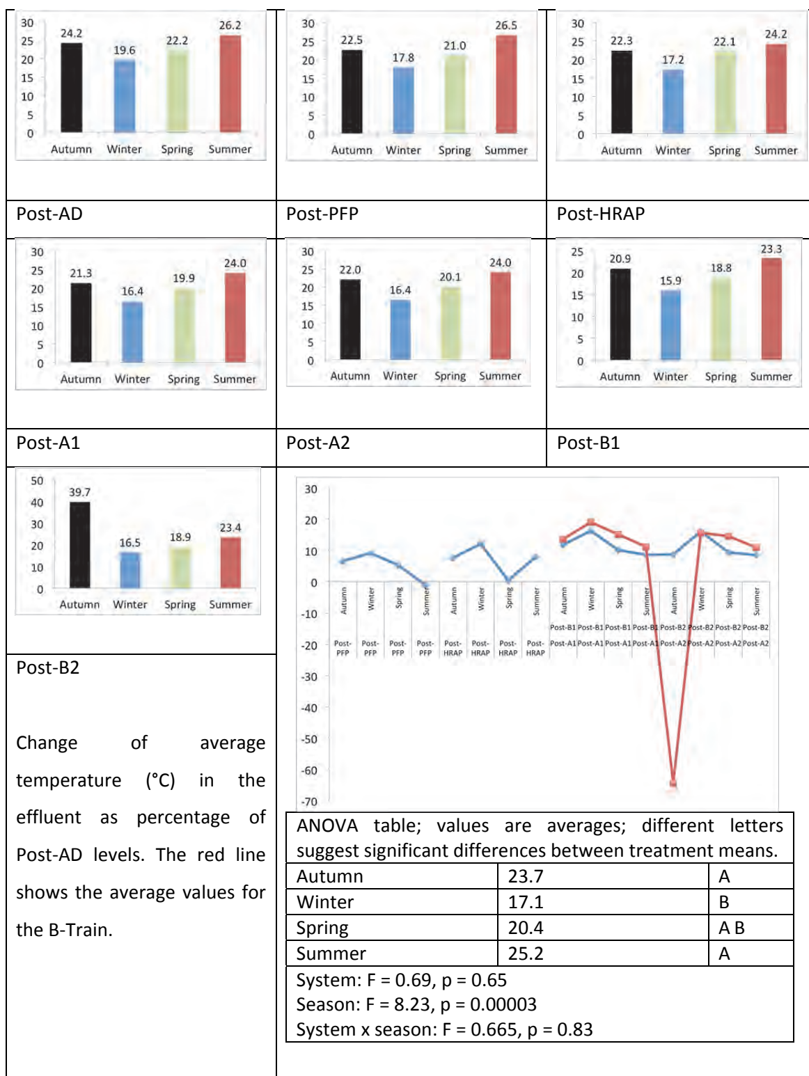
Figure 1.8 Change of average temperature (°C) in the effluent as percentage of Post-AD levels.
