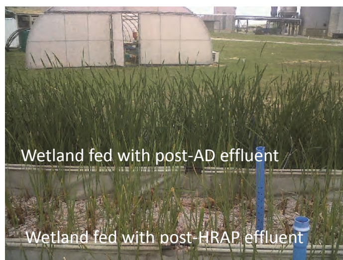
Figure 5.2.1 Reed growth in two constructed wetlands; one fed with effluent from the anaerobic digester (AD) via the primary facultative pond, and one fed from effluent that was first treated in the high rate algal ponding (HRAP) system. The picture was taken on 15 April 2011 (Photo: Lara Crous).
