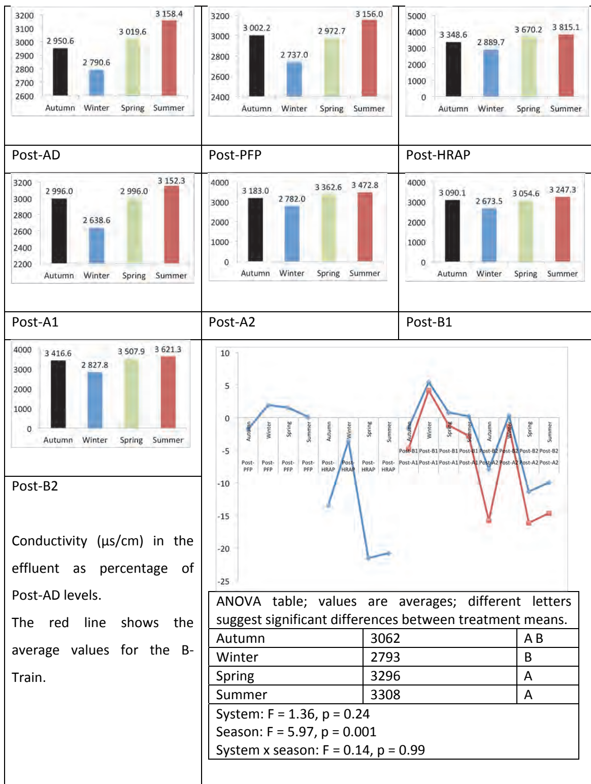
Figure 1.11 Change of conductivity ( \mu\text{s/cm} ) in the effluent as percentage of Post-AD levels.
