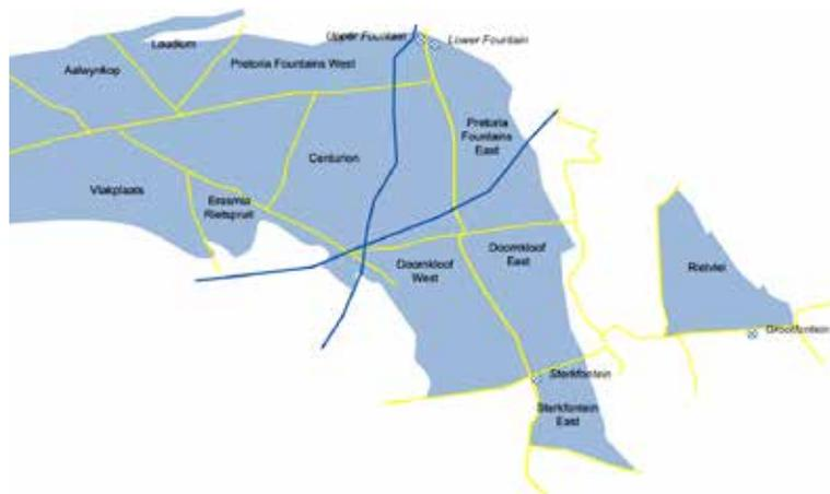
Syenite dykes (indicated in yellow) subdivide the dolomite (indicated in pale blue) into distinct compartments. These dykes may have very low permeability which will limit the amount of interaction between waters in different compartments. They also have a significant influence in the occurrence of springs in the karst areas. Major roads (N1/N14) are indicated in blue (adapted from Holland).
