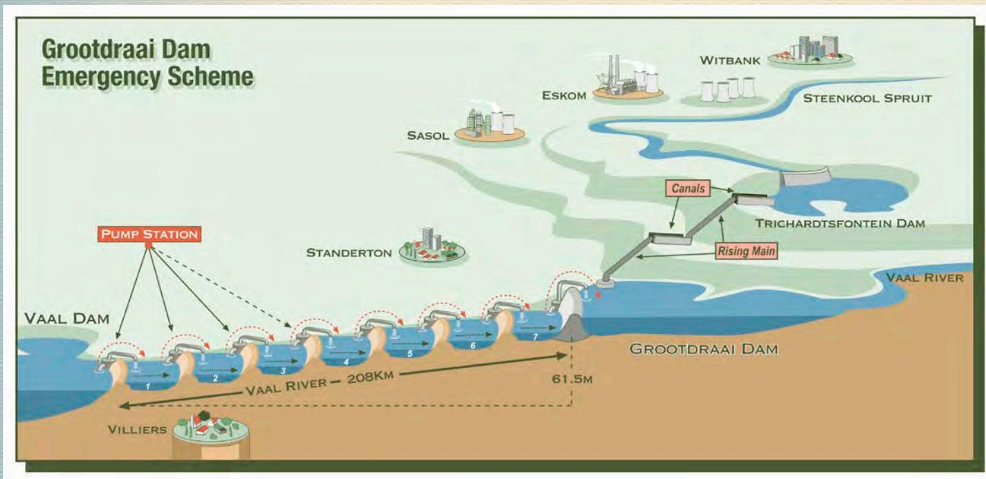
The Grootdraai Emergency Scheme. This scheme effectively reversed the flow of the Vaal River.
