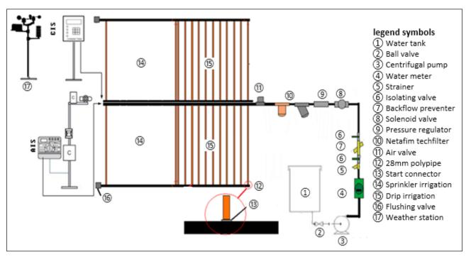
**Figure 1** Schematic design of the experimental field (not to scale)
