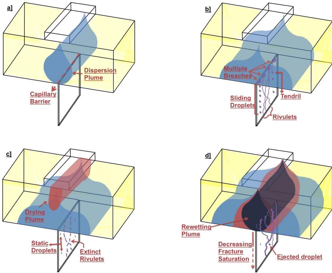
Figure 14-1. Conceptual model for variably saturated flow from soil into a discrete fracture.
