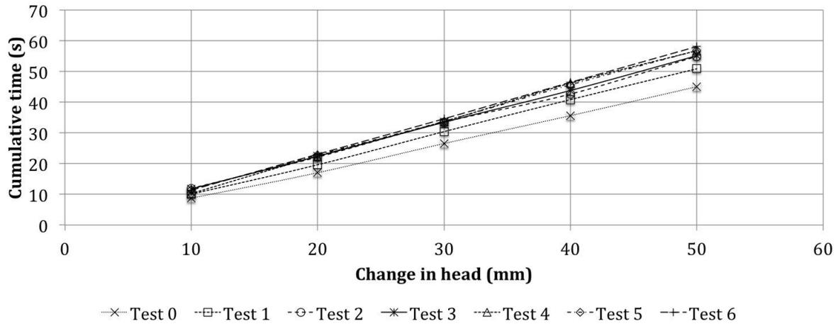
Figure 16-6. Double ring infiltration test results: Welmoed Cemetery.
