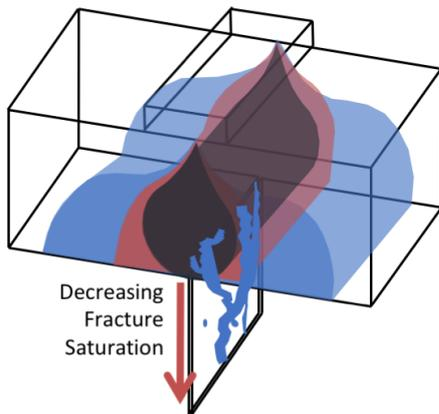
**(b) Unsaturated Flow between Soil and Fractured Rock**
