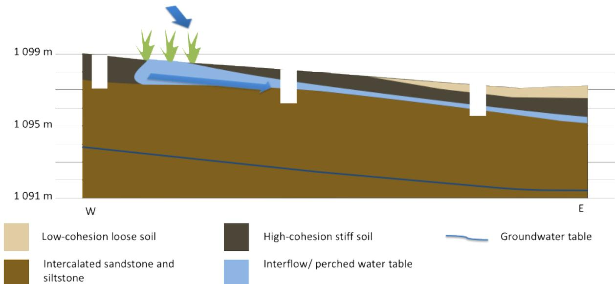
Figure 4-1. Conceptual model of the throughflow system at VZSA3 (Temba, Dippenaar et al., 2014; Dippenaar, 2014).
