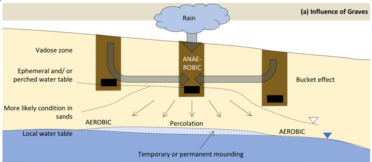
The groundwater table is affected through a so-called bucket effect, whereby graves can act as preferential infiltration zones due to their poorer compaction in comparison to the natural soils. Water will then flood the backfilled graves, from where percolation is promoted to the deeper subsurface.
