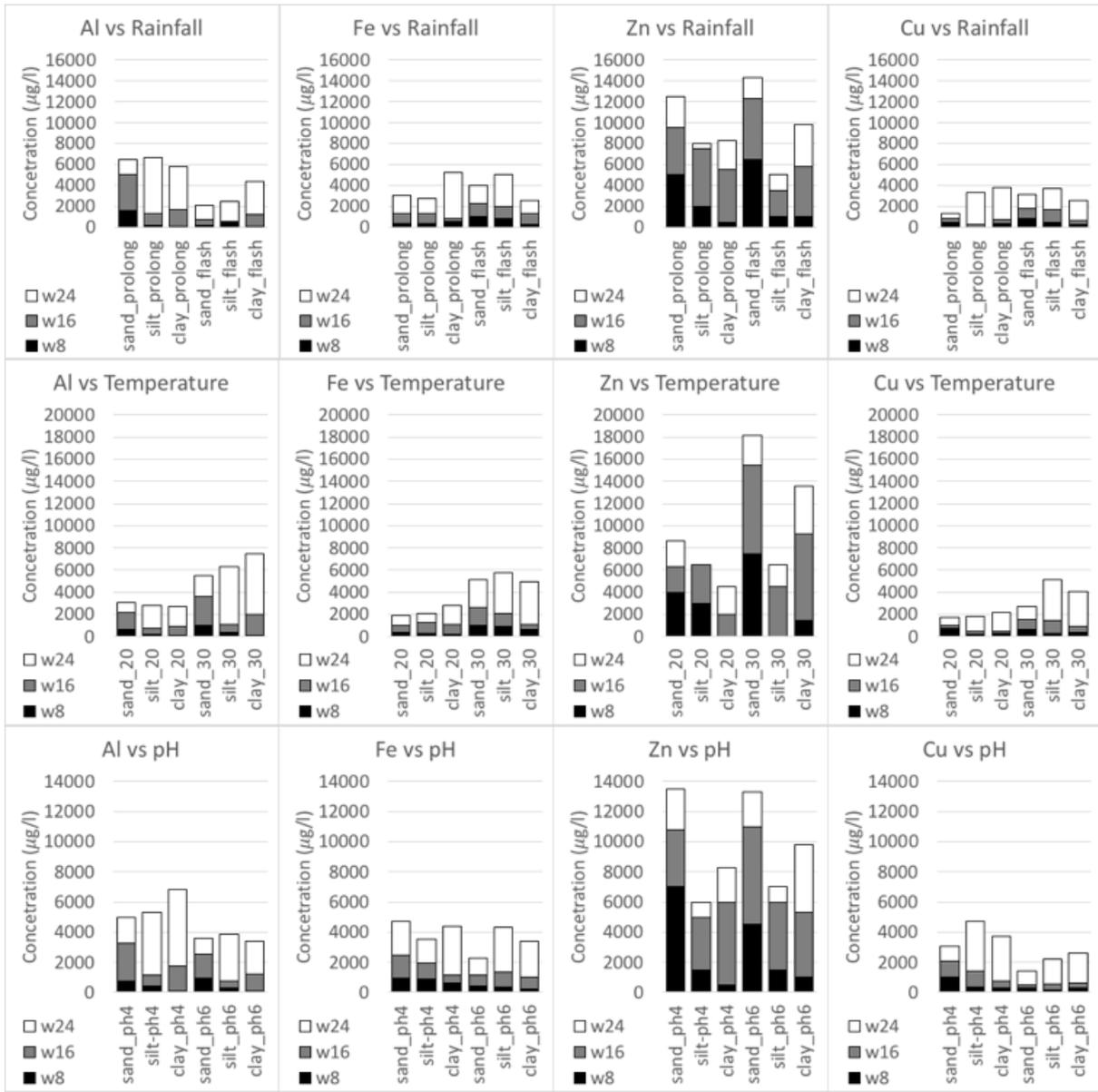
Figure 5-1. Aluminium, iron, zinc and copper leached from the sample columns at week 8, 16 and 24 at different temperatures, rainfall intensities, and pH values (VZSA4, §13).
