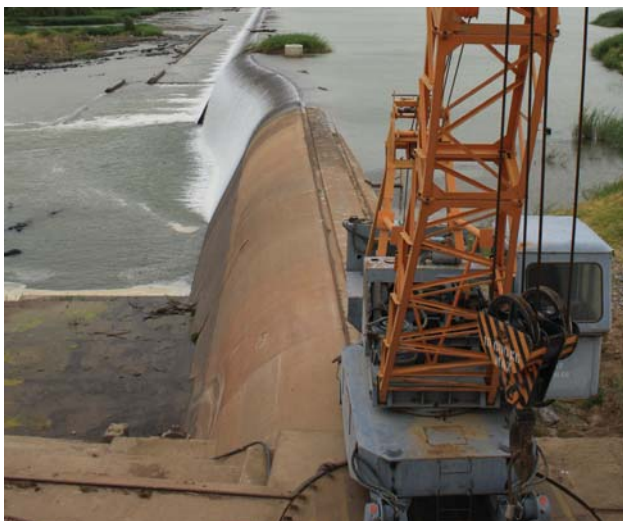
The old crane used to open the dam's 68 sluices.
