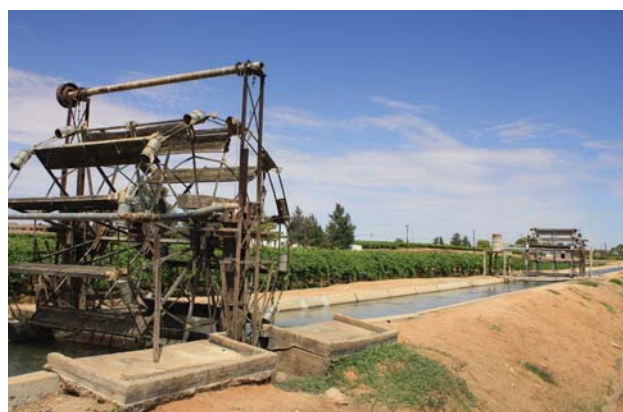
The old water wheels at Kakamas contain small buckets that move water between irrigation canals.
