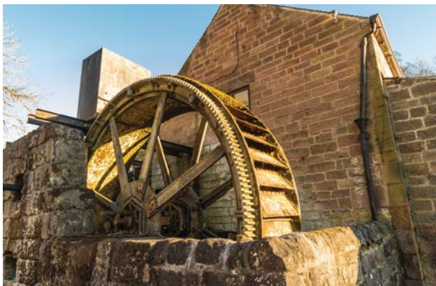
This example of an overshot water wheel can be found in Derbyshire, England.
