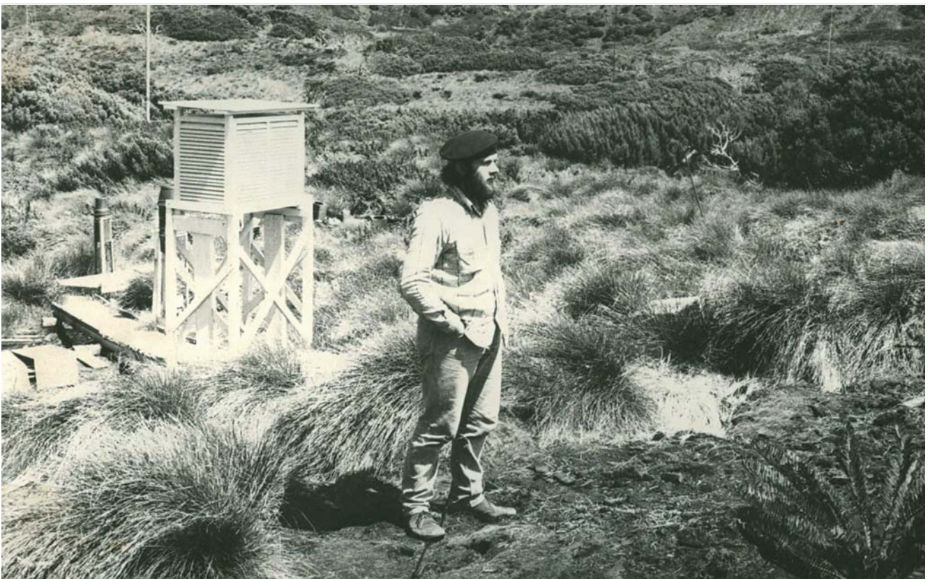
Inspecting the Stevenson screen in 1978.
